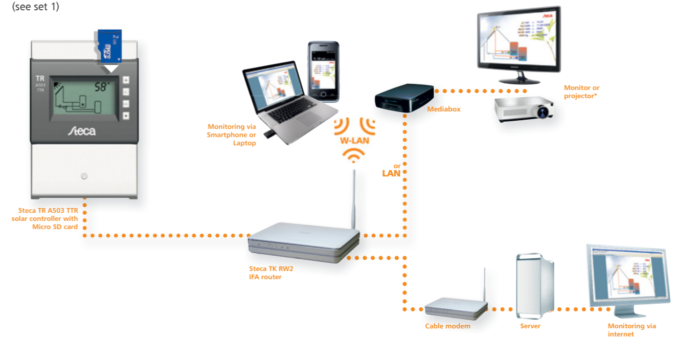
Steca TR A503 TTR solar controller with the Steca TK RW2 IFA router, several WLAN clients and an internet connection (see set 1)
